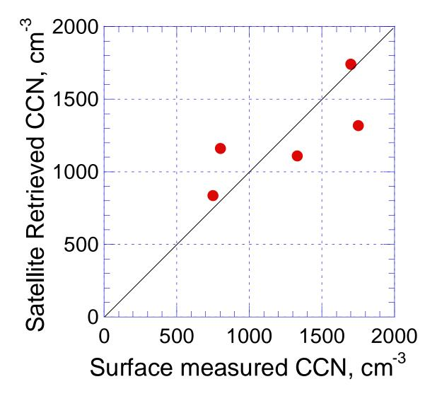
Validation of the satellite-retrieved CCN by surface measurements at the SGP for the 9, 13, 19, 24 and 25 of July 2012. The median  $r_e$  for a given T was used.
