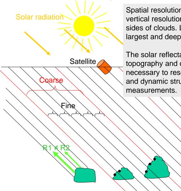
Spatial resolution of ~100 m is required for same vertical resolution from reflectance from vertical sides of clouds. Lower resolution misses all but largest and deepest clouds.
