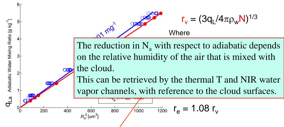
If T-r<sub>e</sub> is so tight, it means that mixing with ambient dry air does not change much  $r_e$ , and it is similar to  $r_e$  of an unmixed (adiabatic) cloud.
